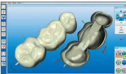
Fig. 6: Milling preview of the veneer and framework structure.
