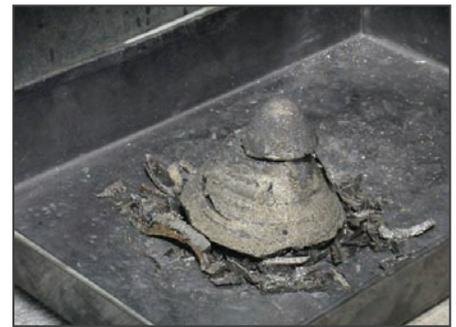
Fig 2: The waste is ground down melted with flux and allowed to solidify. Note the "slag" on the upper surface of the solid mass.
